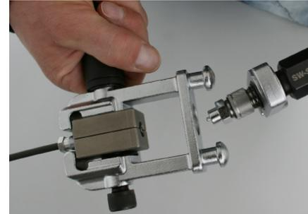
Now screw the pressure spindle (4) together with the pressure piece into the counter-pressure body (2).
