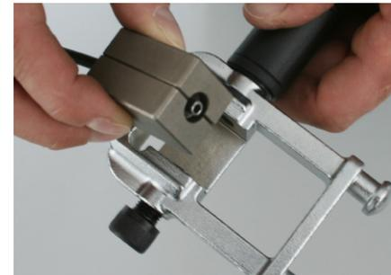
Use the clamping jaws to create the desired flanging edge (90° or 45°).
