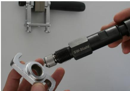
Now turn the counter pressure plate (2) loosely onto the spindle.
