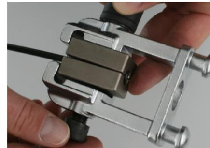
Actuate the clamping screw to clamp the brake hose firmly in the clamping jaws.
