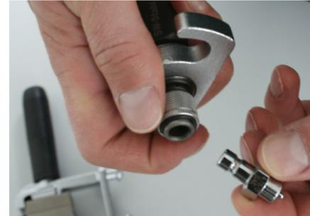
Take the pressure spindle (3) and insert the pressure piece (9 - 13) required for the corresponding flare.
