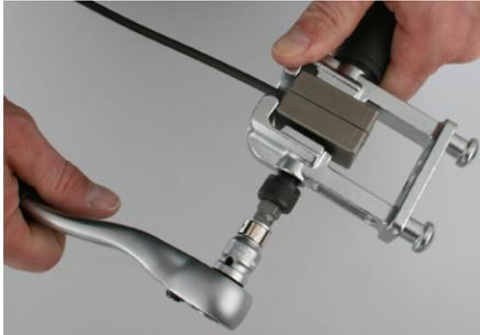
Use a ratchet to press against the jaw firmly to clamp the cable tightly.
