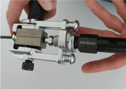
Use the rotary handle (4) to operate the pressure spindle (3) and turn it clockwise until you feel a counter-pressure to complete the flanging.
