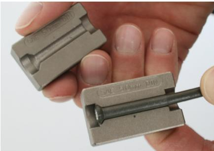
Now turn the rotary handle (4) anti-clockwise to release the pressure piece, then unscrew the pressure spindle (3) completely from the counter-pressure body (2).
